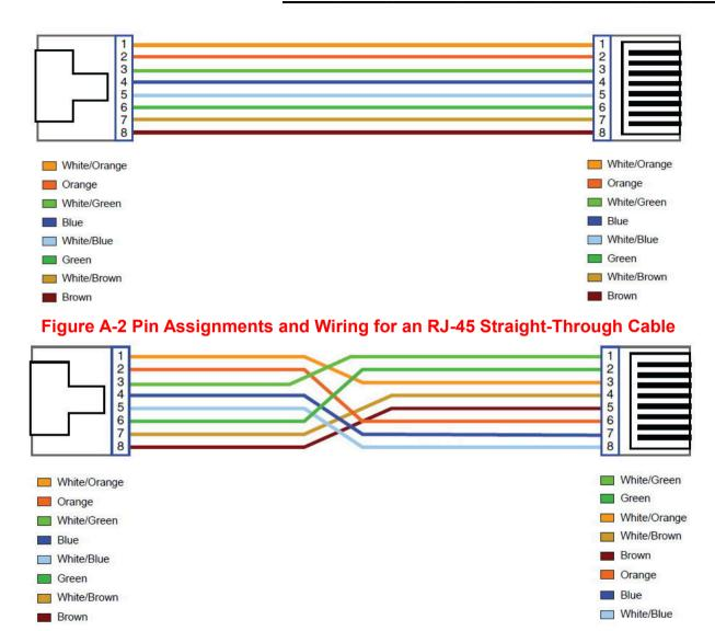
Figure A-3 Pin Assignments and Wiring for an RJ-45 Crossover Cable
