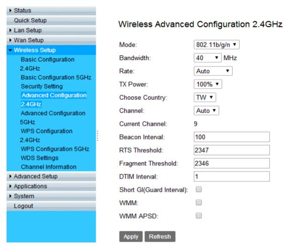
Figure 4.5.1.1 Advanced Configuration 2.4GHz Options
