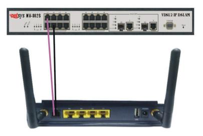
Figure 2.1 NV-720D line ports straight connection
