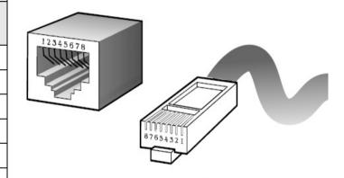
Figure A-1 Standard RJ-45 receptacle/connector
