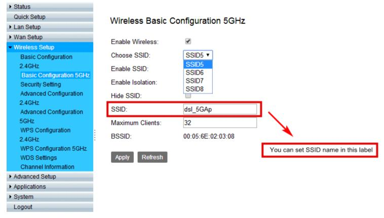
Figure 4.5.2 Basic Configuration 5GHz
